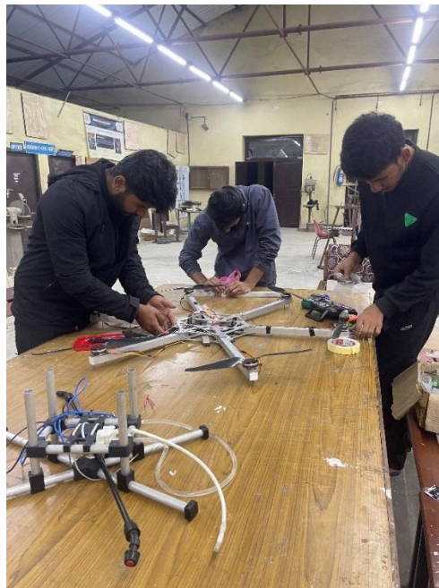
Figure 81: Members Fabricating Drone Frame
